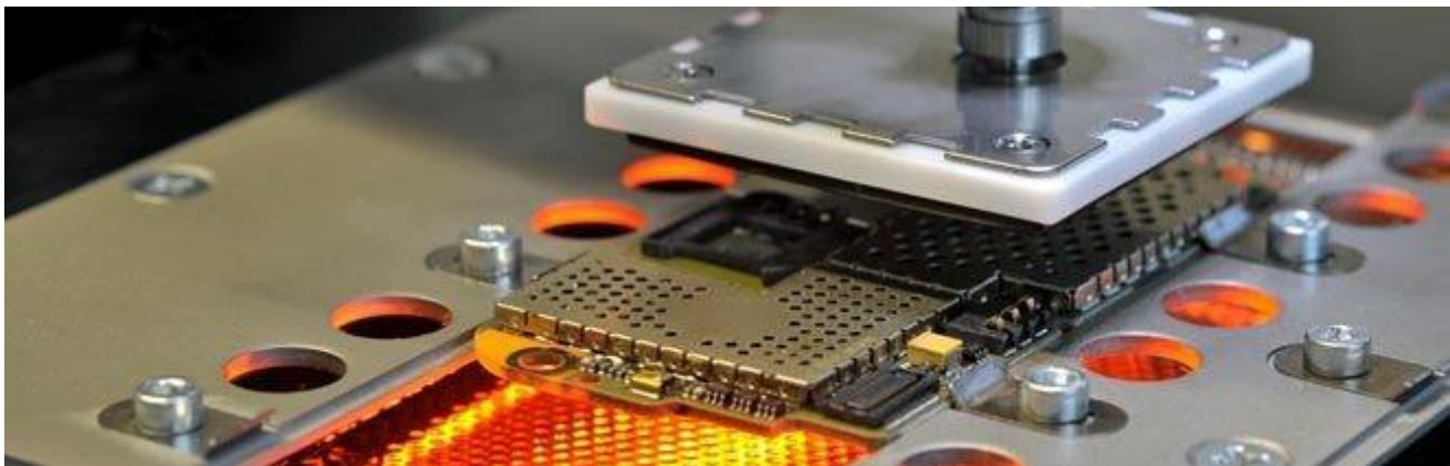
Rework of a shielding frame on a mobile phone
