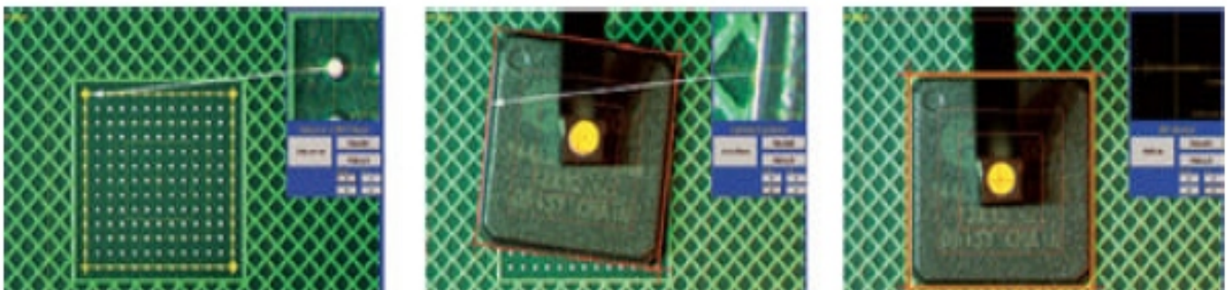
How the AVP works: precise establishing of the target area (left), continuous monitoring (middle) and controlled placement (right).
