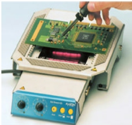
The new underheater Hot-Beam-03
